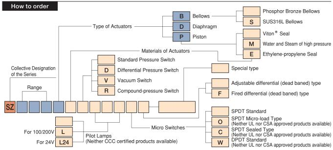
Note: A pilot lamp can not be installed to the DPDT micro switch (type symbol: W).
