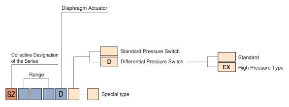
When CCC certified is needed, add appendix of – C to the end of model numbers. Example: An certified of SZ1.7D  $\cdot$  · · · · SZ01.7D-C
