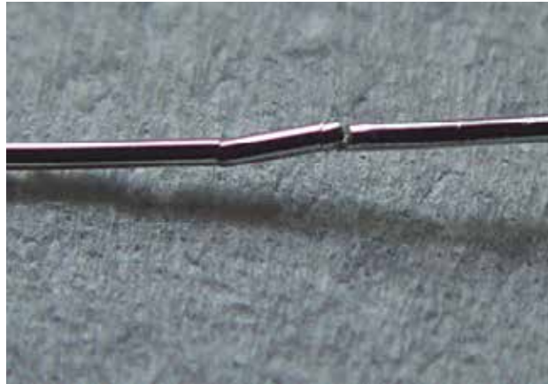
Image 14 - Crystallographic planes slippage
