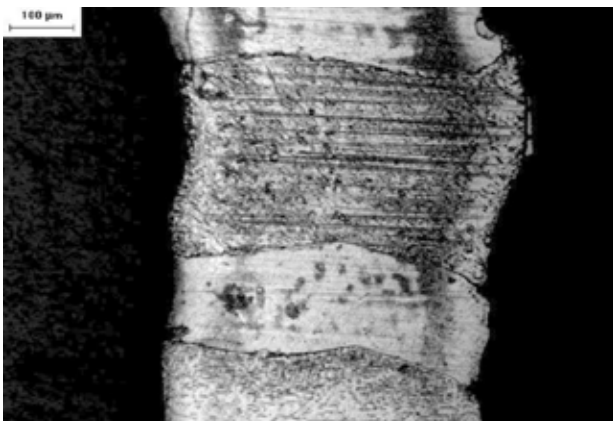
Image 11 - Longitudinal section of a standard Pt wire after 18 months in process
