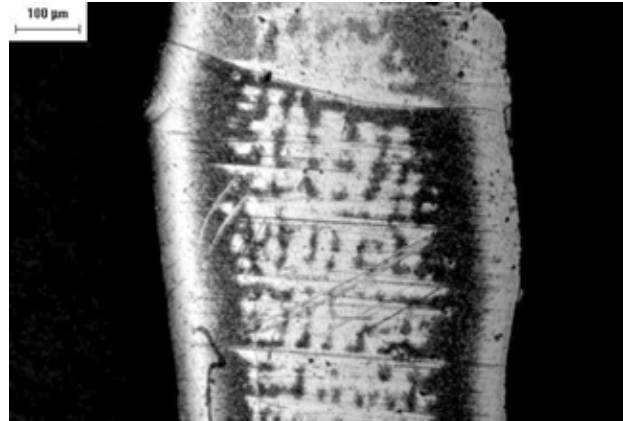
Image 12 - Longitudinal section of a standard Pt wire after 18 months in process
