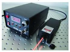
Wavelength 671 nm Operating longitudinal mode Several/one (forSLM) > 100:1 Polarization ratio Point stability < 0.05 mrad Expected lifetime 10 000 hours
