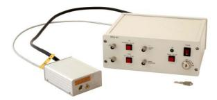
Wavelength 1064 nm Pulse Energy  $70~\mu J$ Pulse Width (FWHM) 0.9 - 3 nsRepetition Rate Timing Jitter (PtP) ≤350 ps
