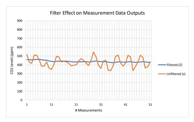
The graph above shows the effects of the filter on the  $CO_2$  measurement data (Z). The unfiltered output (z) is shown in orange and the filtered output (Z) shown in blue.
