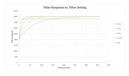
The graph above shows the effect of the filter on response times. Increasing the filter setting increases the measurement output response time.  $T_{90}$  is the time to 90% of reading. The SprintIR<sup>®</sup>-6S takes 20 readings per second. The flow rate was set at 0.2l/min.
