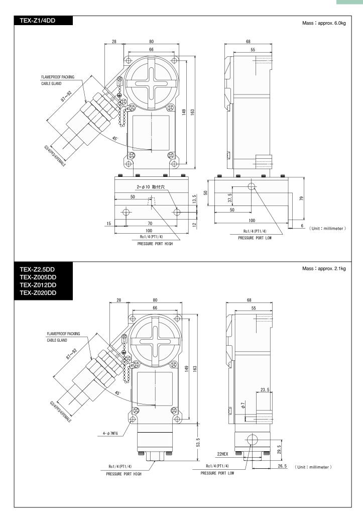
TEX-Z2.5DDEX Mass: approx. 2.5kg TEX-Z005DDEX TEX-Z012DDEX TEX-Z035DDEX 68 80 66 55 FLAMEPROOF PACKING CABLE GLAND 149 MOUNTING SPACER (ACCESSORIES) 0.D. = φ 12 I.D. = φ 8 THICKNESS = 5mm 23. 5 133 12. 4-φ7MTG a P A 62 38 Rc1/4 (PT1/4) Rc1/4 (PT1/4) PRESSURE PORT LOW PRESSURE PORT HIGH 29HEX  $\phi$  65 -35 ( Unit: millimeter )
