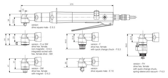
$<sup>\</sup>ensuremath{^{*}}\xspace$  ) Measurement plus length of bit or sockets is space requirement.
