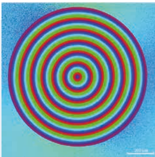
Fast axis distribution across the element (measured with HINDS MicroImager)
