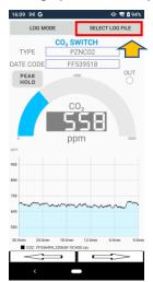
⑤ Press the button of "PEAK HOLD" to visible the highest concentration value. Repress the button of "PEAK HOLD" to be cleared.
