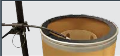
Top view of turn table showing wire guide and wire retainer ring
