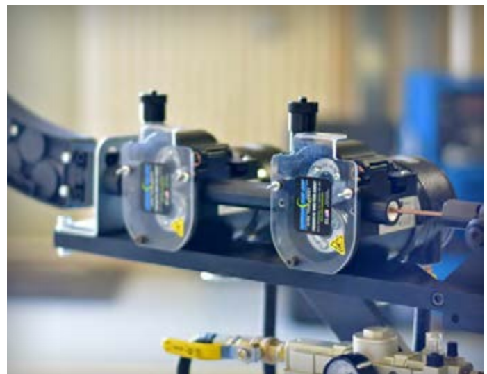
Tandem Wire Feed Assists Installed on a Mechanical Turn Table.
