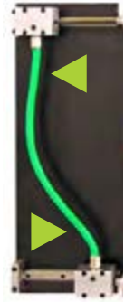
Flexural Strength Testing Device
