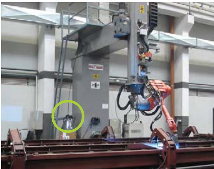
Wire Feed Assist installed in a robotic gantry application.
