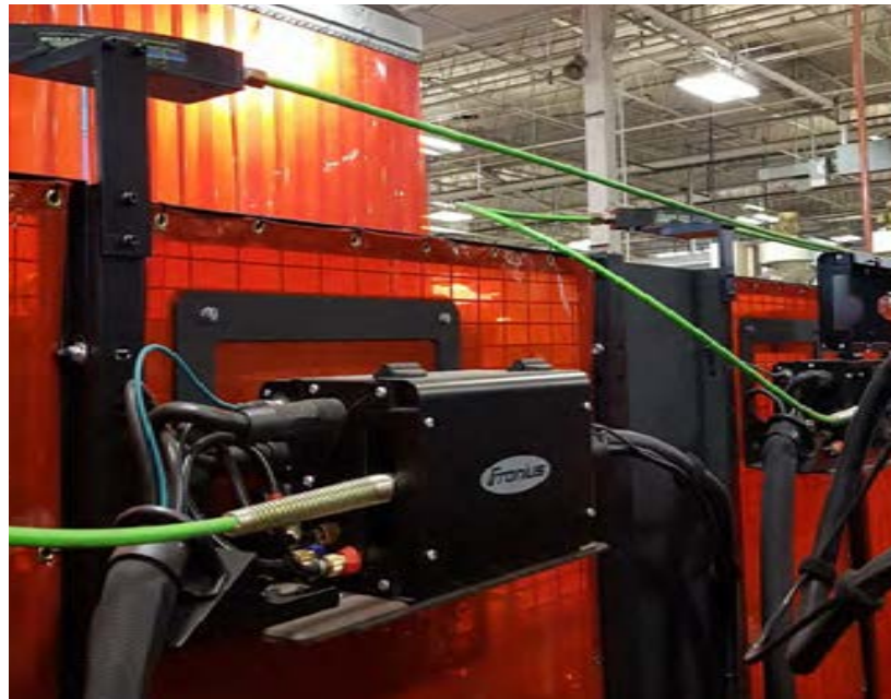
Wire Wizard® inlet guides, conduit and Wire Guide Modules were installed in this optimized wire delivery setup with wire feeders mounted in a fixed position outside the weld cell.
